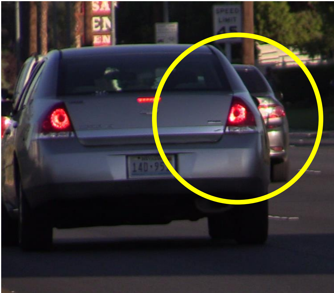
Figure 3-24. Occlusion of vehicle in Lane 2 by vehicle in Lane 1 at Site 2
